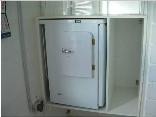
A thermocabinet running at 17°C for delivery of AI
